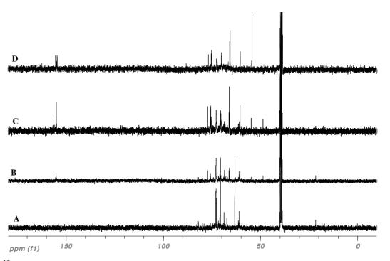
**Figure 5:** <sup>13</sup>C NMR of the reaction product between PG3 and different amounts of CDM (A) PG3 (B), PG3 with 1équivalent CDM (C), PG3 with 3 equivalents of CDM (D), with 10 equivalents of CDM
