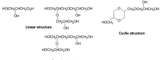
Branched structures Figure 2: Different isomers of PG3
