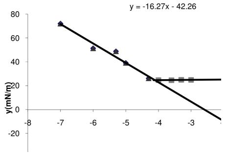
Figure 7: Changes in surface tension as a function of concentration
