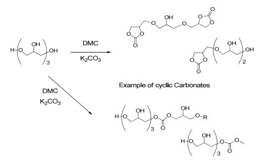
**Example of acyclic Carbonates Figure 3:** Some examples of reactions in the group of carbonate formation.
